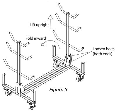
3. Tighten the 2 lower bolts that are captured in the upright support to prevent the folded uprights from bouncing or otherwise moving during transport. (See Dis-Assembly Figure 4).
