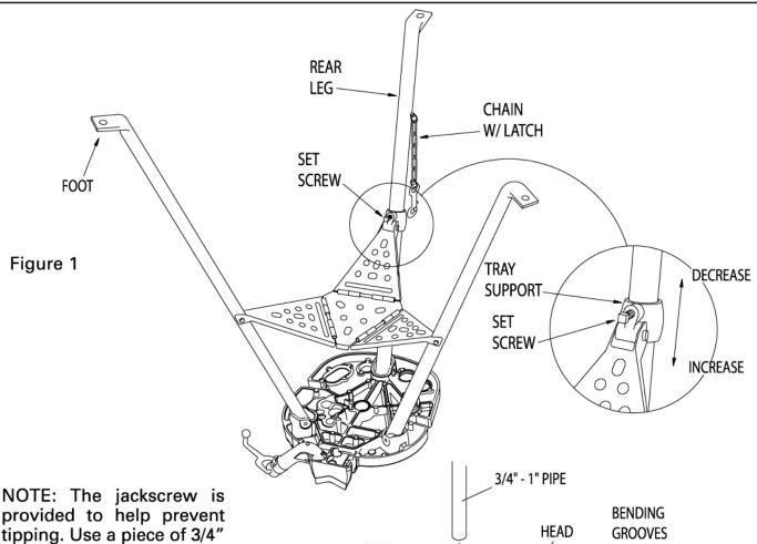
NOTE: The jackscrew is provided to help prevent tipping. Use a piece of 3/4" or 1" pipe as a brace against the ceiling to help anchor the Chain Vise Stand. Be sure the ceiling is capable of supporting the load that will be placed against it.
