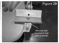
2. The two lower jaws are installed on the base of the stand (see Figure 2A) using the two lower jaw screws removed in Step 1. The notched side of the two lower jaws are installed to the high side (see Figure 2B). Then, install the upper jaw in the yoke assembly. Be sure the upper jaw is flush with the jaw
